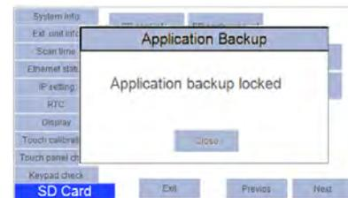
5. If free size on SD card is not sufficient to copy application program, then device will block backup process with error message as shown below.
