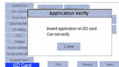
7. During verification, device checks application program and all supporting files on device and SD card.
