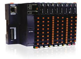
Modular I/O series is ideal for application requiring flexible and cost-effective remote I/Os. Modular I/O station can be formed by using required Header module, I/O modules and System modules required for it.
