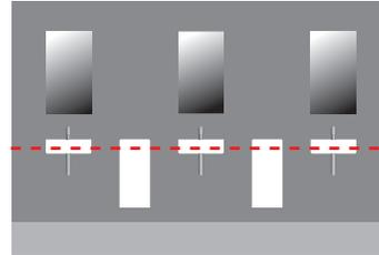
Install multiple units neatly aligned with sinks.
