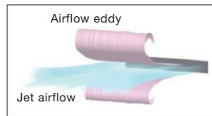
Eddy generated with straight nozzle outlet flows easily, becoming a source of noise.
