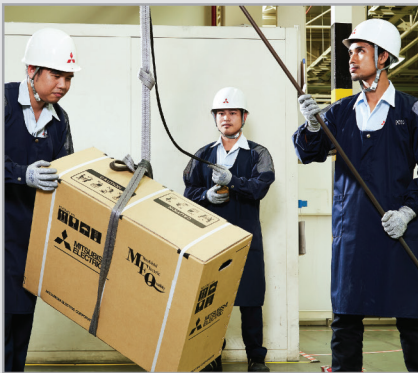
DROPPING TEST Performed to confirm its packing quality can withstand heavy handling and repeated transportation.
