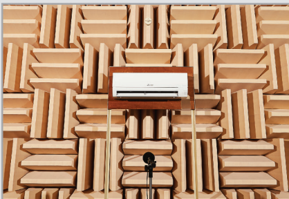
ANECHOIC CHAMBER NOISE TEST Performed for sound pressure level & power pressure level
