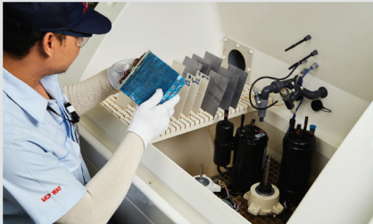
SALT SPRAY TEST Performed to control metal part quality
